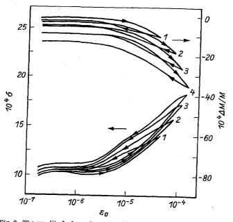
Fig. 2. The amplitude dependences of  $\delta$  and  $\Delta M/M$  in bismuth at 300 K
