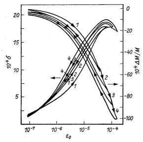
Fig. 1. The amplitude dependences of decrement (left axis) and modulus defect (right axis) in bismuth at 6 K. The figures indicate numbers of the successive measurement runs at which the maximum measurement amplitude is gradually increased
