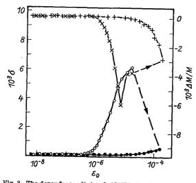
Fig. 3. The dependences  $\delta(\varepsilon_0)$  and  $\Delta M/M(\varepsilon_0)$  in the antimony single crystals of the orientation I at 300 K. O,  $\times$  – direct runs,  $\bullet$ , + – reverse runs
